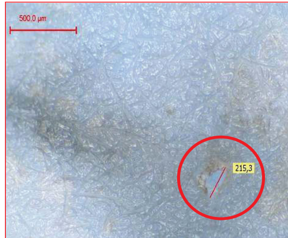
Burn hole in the filter material
