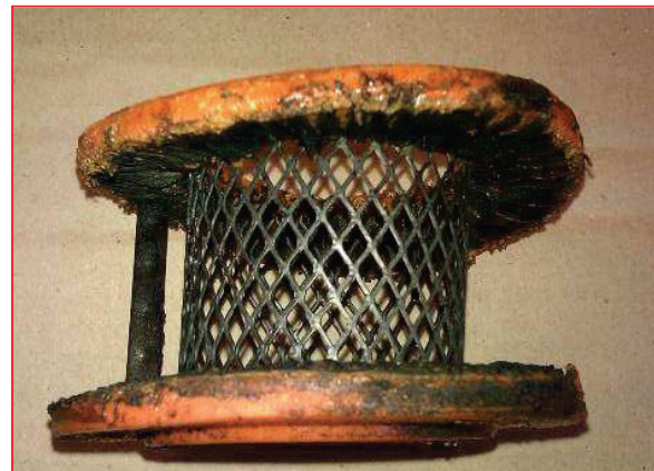
Breather filter burned as a result of explosion in the tank
